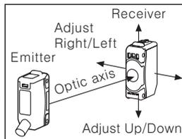
※ When the sensing target is translucent or small (Under  $\phi$  16mm), it can be missed by the sensor because the light can penetrate it.
