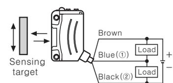
※① : The load connection of NPN open collector output, ② : The load connection of PNP open collector output
