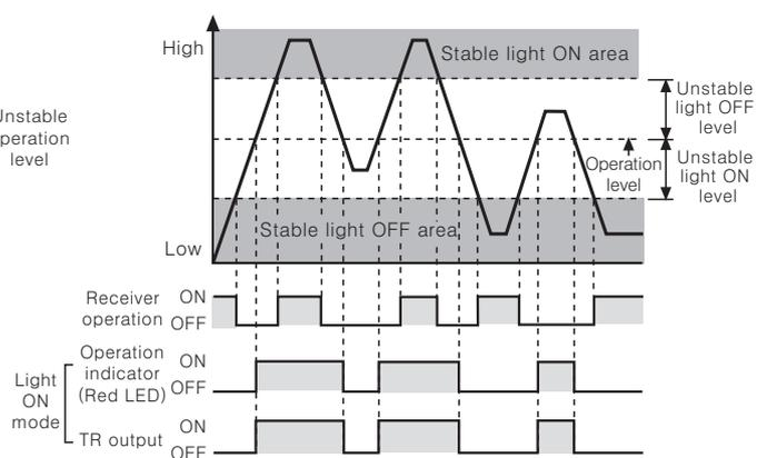
※ The waveform of 'Operation mode indicator' and 'TR output' is for Light ON mode, it is operated as reverse in Dark ON mode.
